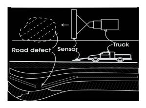
Previously there has been no practical way to monitor the condition of the earth supporting the infrastructure. We have invented a "smart" material which can be embedded underground during construction or reconstruction, and which provides an easy-to-use and inexpensive means to verify the integrity of the underlying earth.
